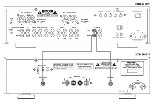
Figure 5: XLR Cable Connections
